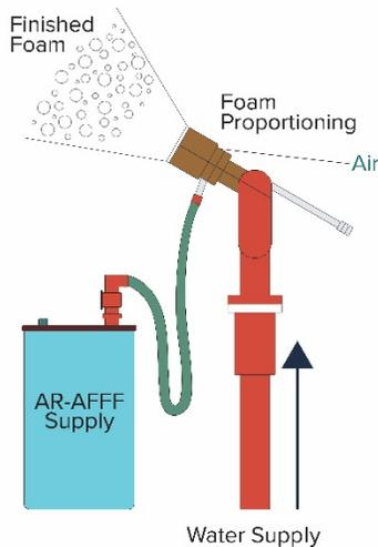
All of these elements must be combined properly to produce a quality finished foam blanket. If any of these elements are missing or are not properly proportioned, the result is a poor-quality foam or no foam at all.
