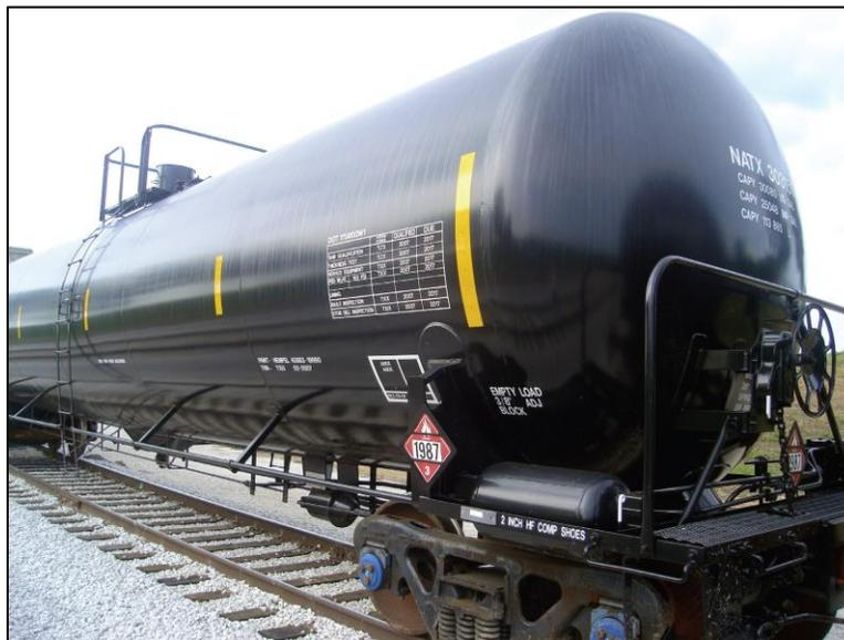
New regulations for rail tank cars construction were published in 2015. New rail tank cars constructed after October 1, 2015 are required to meet enhanced DOT Specification 117 design or performance criteria. Existing rail tank cars must be retrofitted by 2023 in accordance with the DOT-prescribed retrofit design or performance standard.
