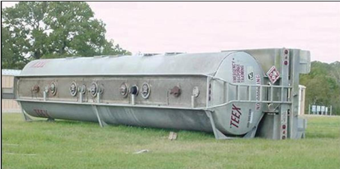
Ethanol transported in cargo tank trucks are placarded and marked in the same manner as all other hazardous materials. Other characteristics of the cargo tank trucks are pressure and vacuum relief devices. They are typically bottom loaded and unloaded and equipped with a vapor recovery system.
